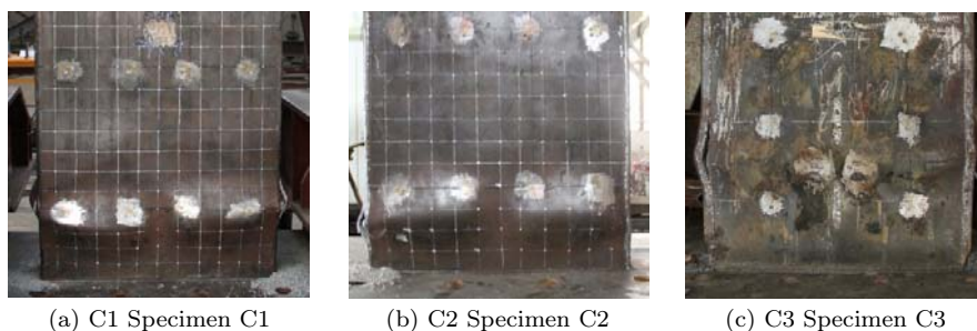
Fig. 5. Failure mode of specimens
